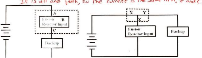
A = entering the reactor B = through the reactor C = leaving the reactor X = entering the junction Y = on the way to the backup from the junction Z = on the way to the reactor from the junction
