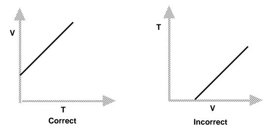
By established convention it is proper to plot V = f(T) rather than T = f(V), since the experimenter can directly control the temperature of the gas, but the volume can only be changed by changing the temperature.
